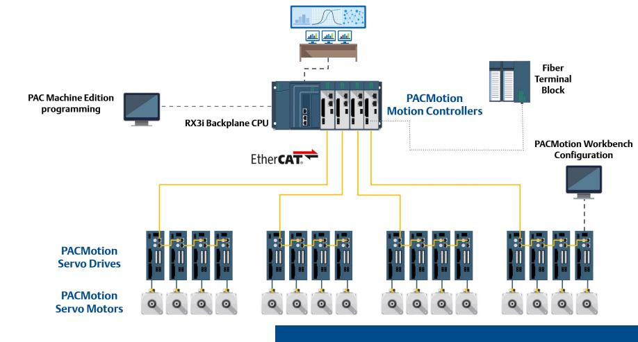
From single point-to-point indexing to complex multi-axis machine control, PACMotion servo solutions provide the flexibility to integrate a system that optimizes performance and investment.
