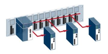
PACMotion is based on PACcore, a multi-core CPU architecture whereby the PAC CPU runs the application program while up to 10 dedicated co-CPUs run the motion algorithms
